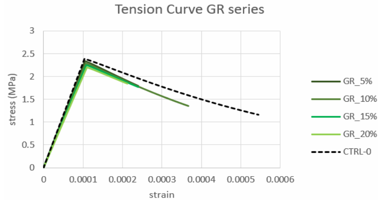
Figure 7. Tensile stress-strain curves for the GR series concretes (5%, 10%, 15%, 20%) compared with the control concrete CTRL-0.
